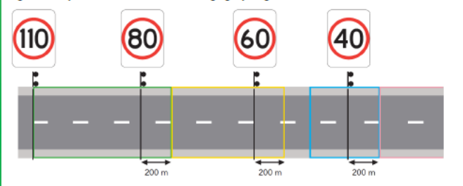
Figure 2.2: Speed to be used for advance warning sign spacing
